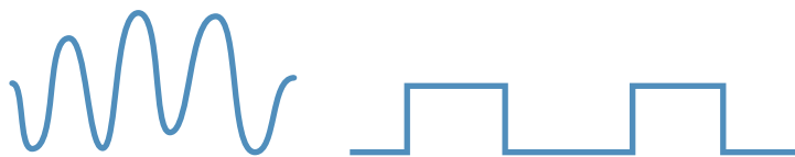
FIGURE 3.2 An analog signal and a digital signal
